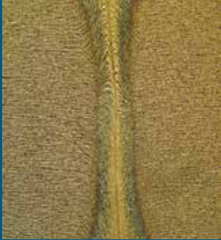
"As welded" microstructure showing weld bond plane and HAZ (Heat Affected Zone) with "hour glass" very evident.
